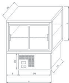
Drop-in Refrigerated Show Case „EUROLINE“ 2 levels, glass shelves, sliding doors, suspended cooling unit
