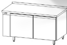
Standard execution – Remote cooling with hinged doors, Technical compartment left side
